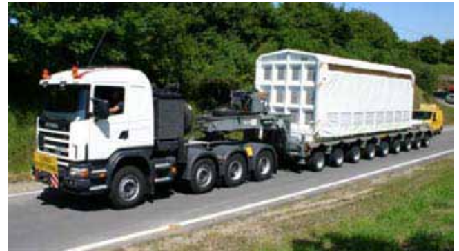
Rail car with a transportation cask used in Europe (top-left); package and trailer for road transport of used nuclear fuel (top-right). Photos from Areva. Ship for used nuclear fuel transport in Sweden (left). Photo from SKB.
