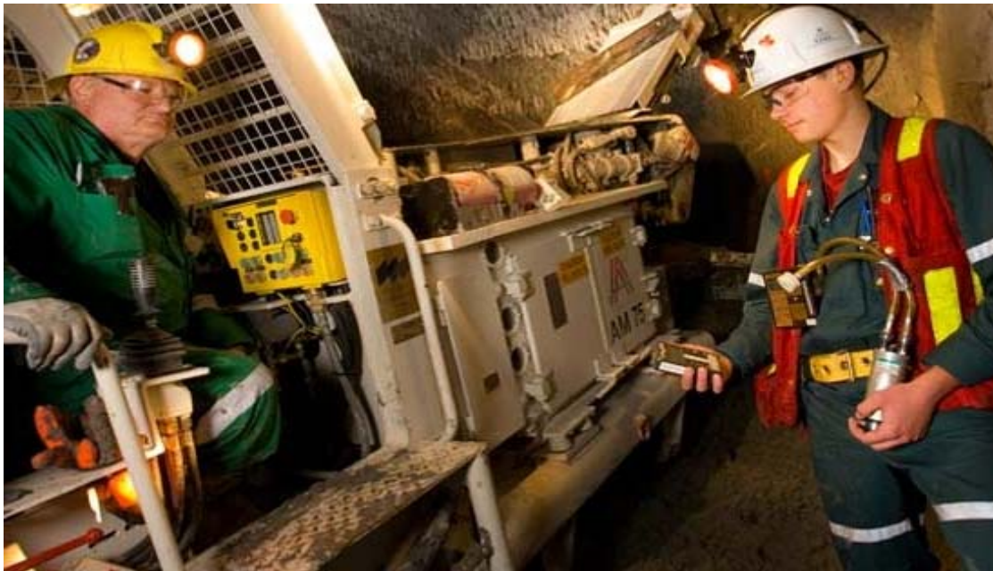
Figure 49: Manual Air Quality Monitoring
