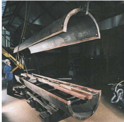
Figure A-2: Assembly of Tube Halves for Longitudinal Welding
