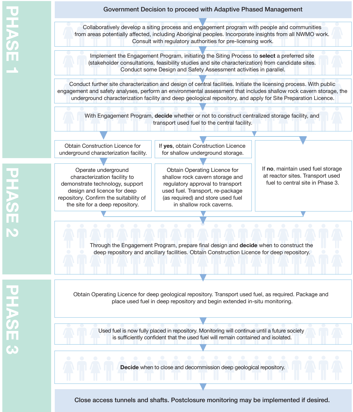
Figure 1-2 Activity Flowchart for Adaptive Phased Management
