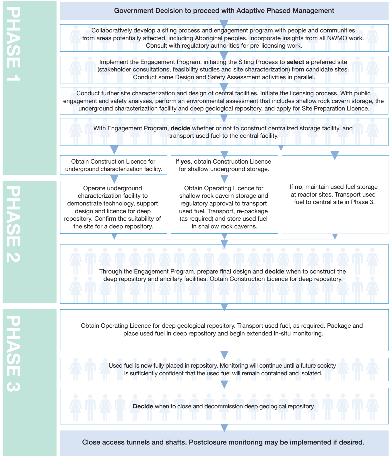
Figure 1-2 Activity Flowchart for Adaptive Phased Management
