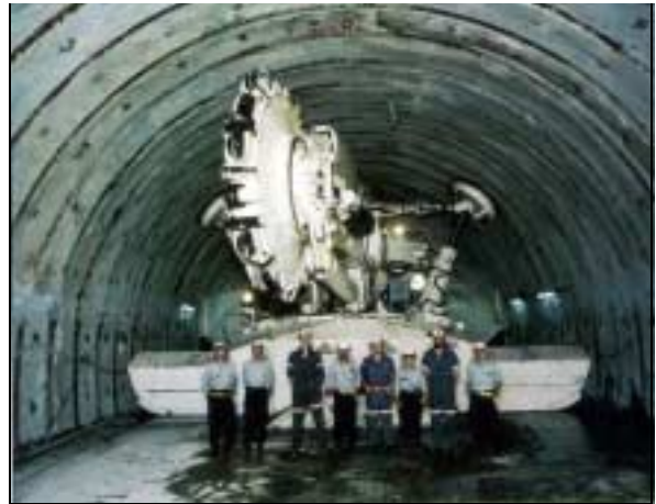
Continuous Mobile Miner, capable of tight (11m) radius turns, good wall profile control and mining non-circular shapes
