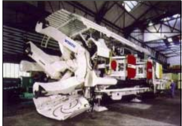
Continuous Mobile Miner, capable of tight (11m) radius turns, good wall profile control and mining non-circular shapes
