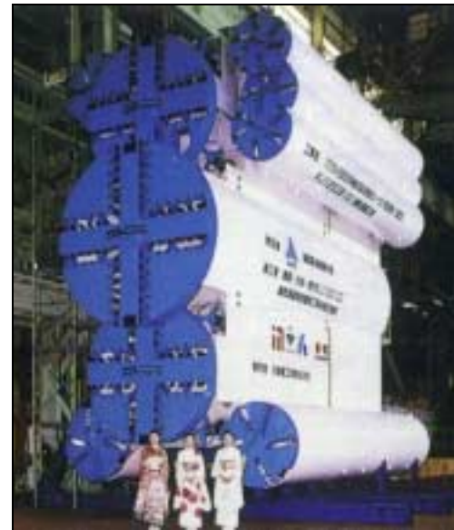
Figure 2 – Various types of esoteric multi-face machines mainly for soft ground excavation. Note: some multi-face prototypes are already in development for hard-rock utilization.
