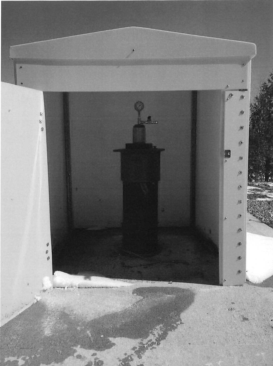
Figure 5: Example of an enclosure placed atop of an instrumented well head.
