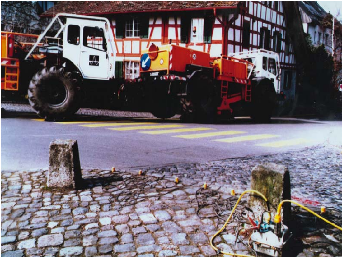
Figure 14: Field investigations to characterise the deep underground commonly include a seismic campaign used to map the geological strata. The illustration shows a heavy vibrator inducing pressure waves that will be reflected at the different geological interfaces. This technique is most successful in layered sedimentary geological structures.
