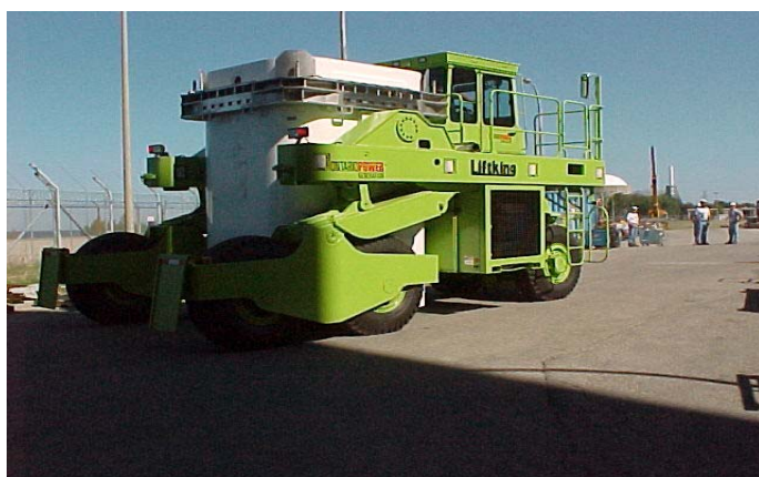
Figure 2.3: Transfer of Dry Storage Canister at Bruce B Ancillary Services Building
