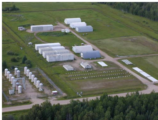
Figure 2.12: Whiteshell Waste Management Area (Dry Storage Cannisters are in the lower left of the Figure)
