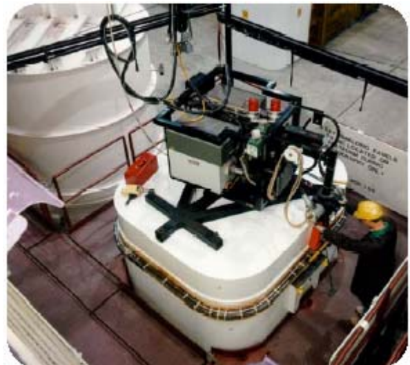
Figure 28. X-ray of weld on DSC (Pickering Waste Management Facility - Phase II Information Package)
