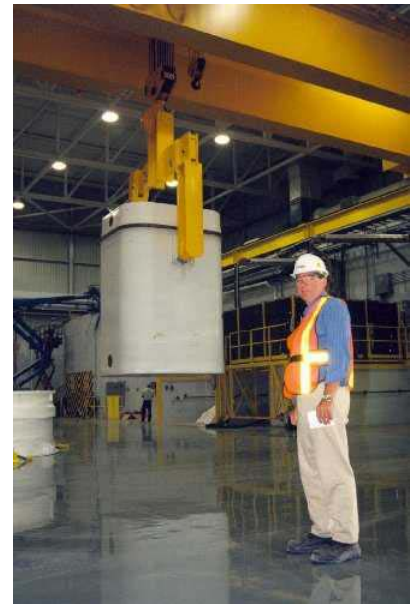
Figure 31. DSC being moved by crane.
