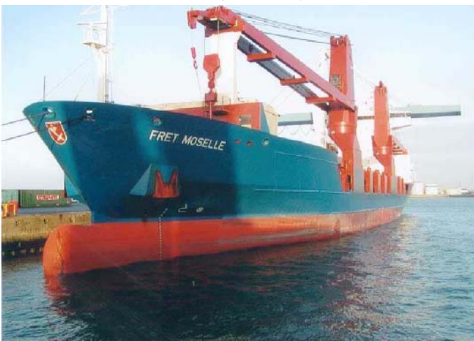
Figure 35. Ship with on-board crane. (Cogema Logistics Ltd.).
