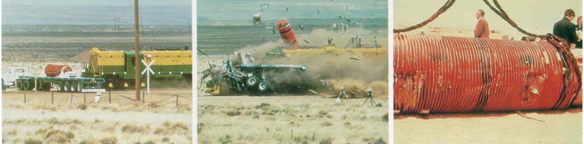
Figure 9. Locomotive Crash test: cask remains intact ( http://www.nuclearfaq.ca/cnf_sectionJ.htm#images )
