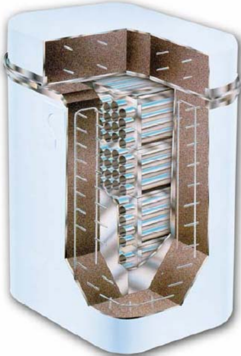
Figure 27. DSC Cross Section (Pickering Waste Management Facility - Phase II Information Package)
