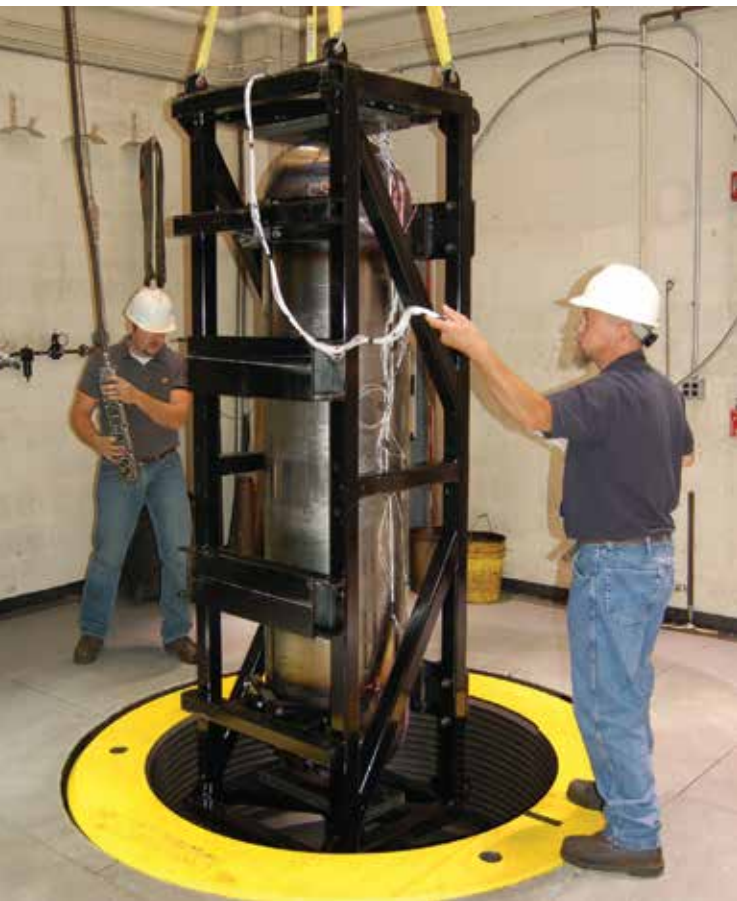
A used fuel container is lowered into the isostatic press at the Applied Research Laboratory's High-Pressure Test Facility at Pennsylvania State University.
