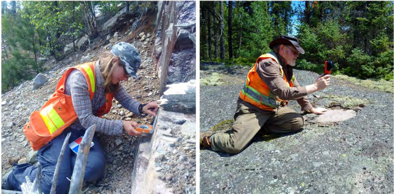
Photograph 2: Example of outcrop measurements (structural orientation of a joint and magnetic susceptibility, respectively), June 6, 2017.
