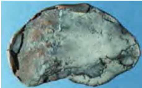
Found in clay-rich mudstone, this 12-centimetre copper plate experienced little-to-no corrosion for 200 million years.
