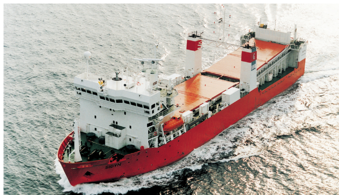
Figure 4: Ship for used fuel transport in Sweden
