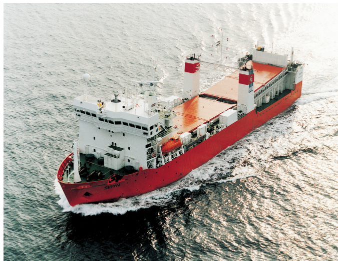
Figure 4: Ship for used fuel transport in Sweden. Photo from SKB.
