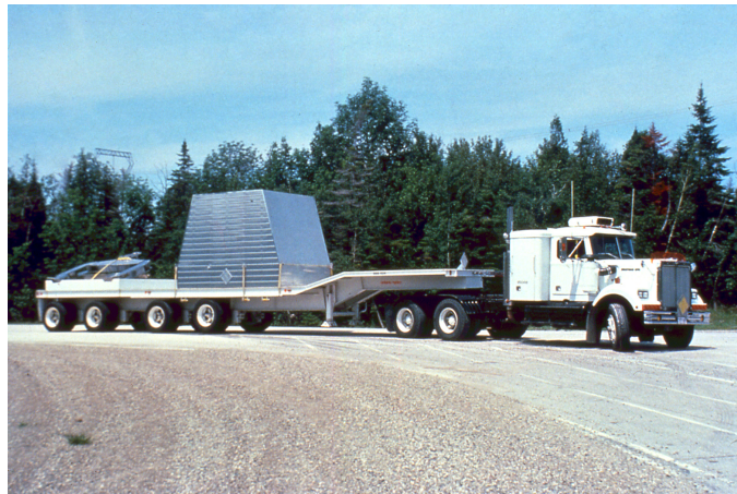
Figure 3: Tractor-trailers for road transport of used fuel: OPG
