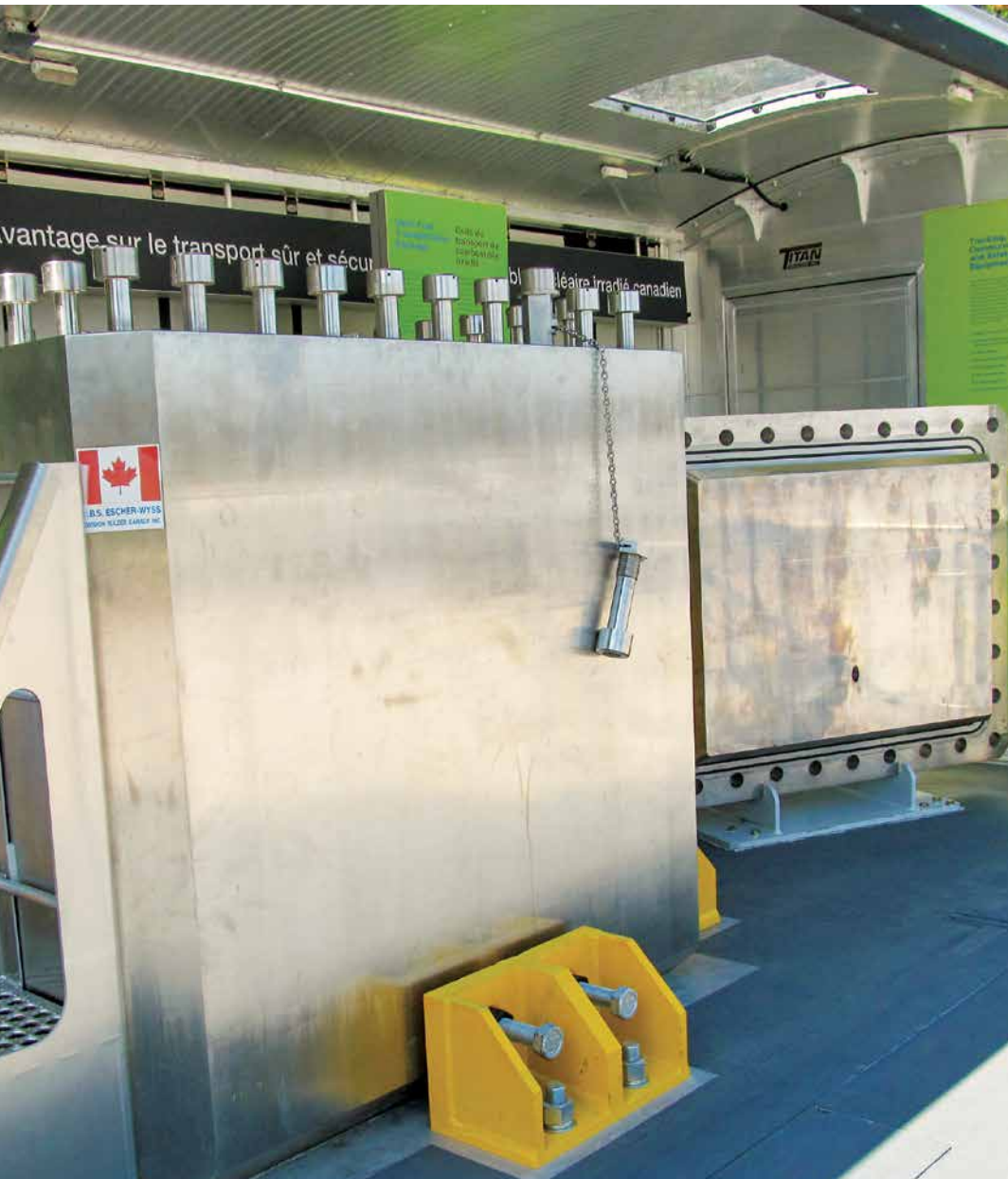
The transportation container, shown here as part of an exhibit, is a solid stainless steel box with walls nearly 30 centimetres thick. It has been safety tested under even the most severe accident conditions.
