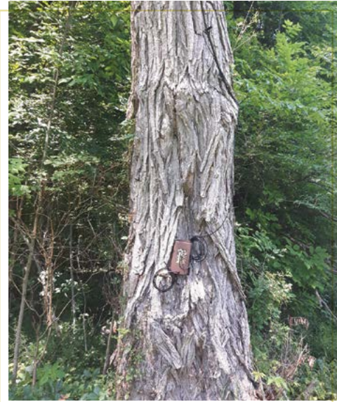
An acoustic monitor is installed in the South Bruce area to identify bats.
