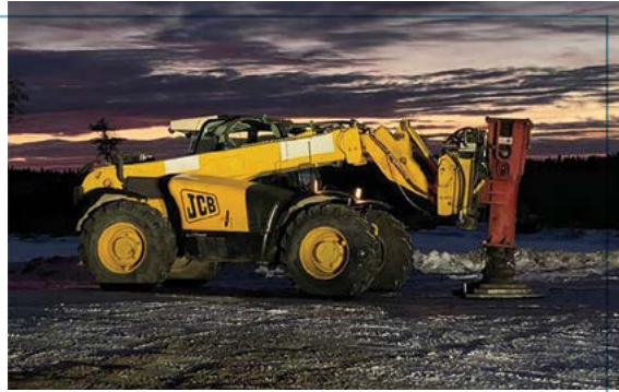
A seismic source vehicle conducted 2D seismic survey in the Ignace area.
