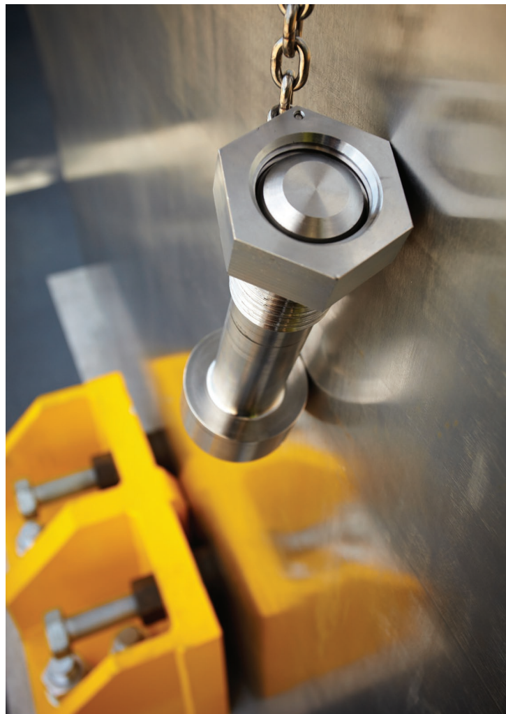
One of 32 bolts that holds the lid of the UFTP in place.
