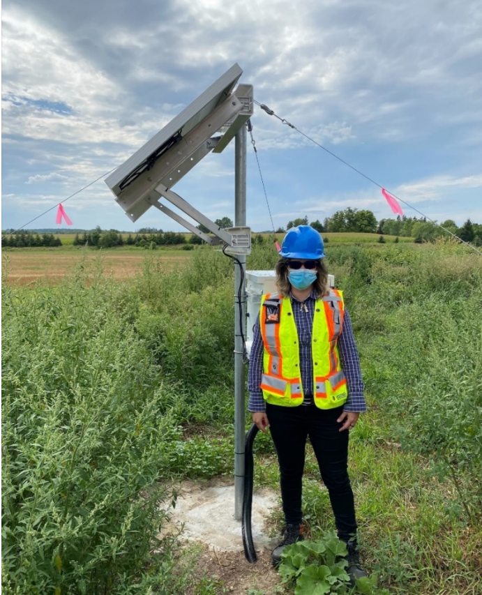
Figure 14.1: Photo of one of five microseismic monitoring stations installed around the area in order to obtain more detailed information on site seismicity.
