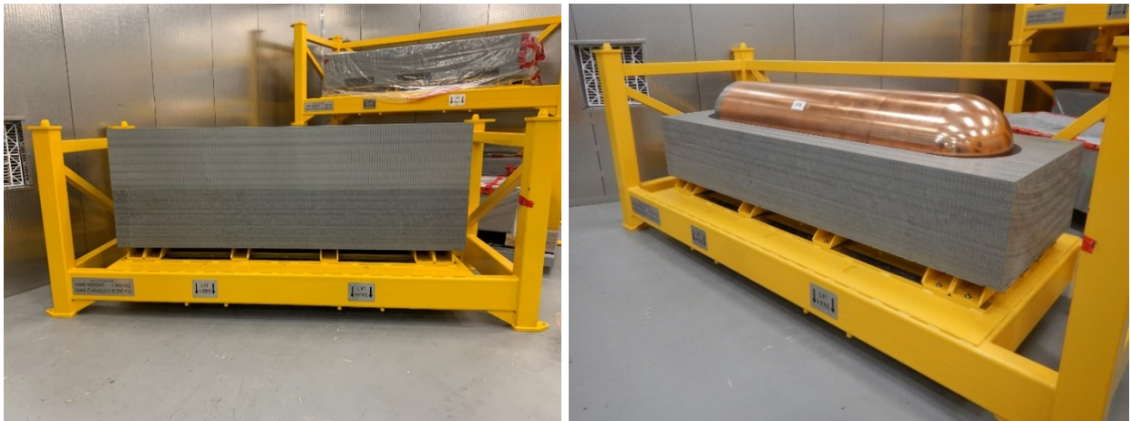
Figure 7.6: Prototype Buffer Box and Used Fuel Container
