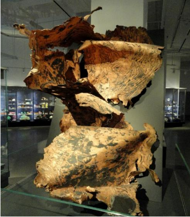
Figure 9.2: Natural copper sheet from White Pine Mine, Keweenaw Peninsula, Michigan, USA (on display at Royal Ontario Museum). This copper shape is because it was extracted by blasting in the mine. The copper sheet is about 1 billion years old.
