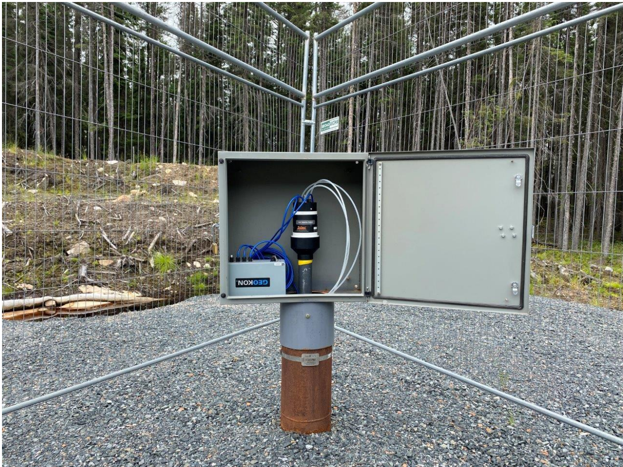
Figure 7-1: Installed shallow groundwater monitoring well in the WLON-Ignace area.
