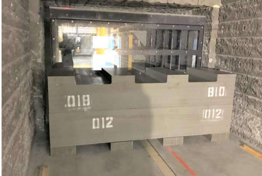
Figure 3-24: Buffer Box 1 Inside Mock Emplacement Room
