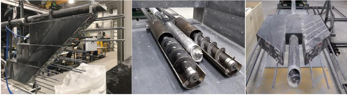
Figure 3-12: Vertical and Horizontal GFM Void Prototypes
