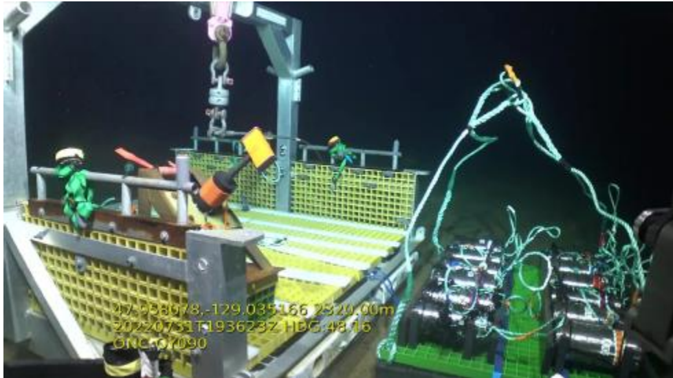
Figure 4-15: Engineered Barrier Testing Modules Deployed on the Floor of the Pacific Ocean at the Endeavour Observatory Operated by Ocean Networks Canada at About 3000 m Depth.
