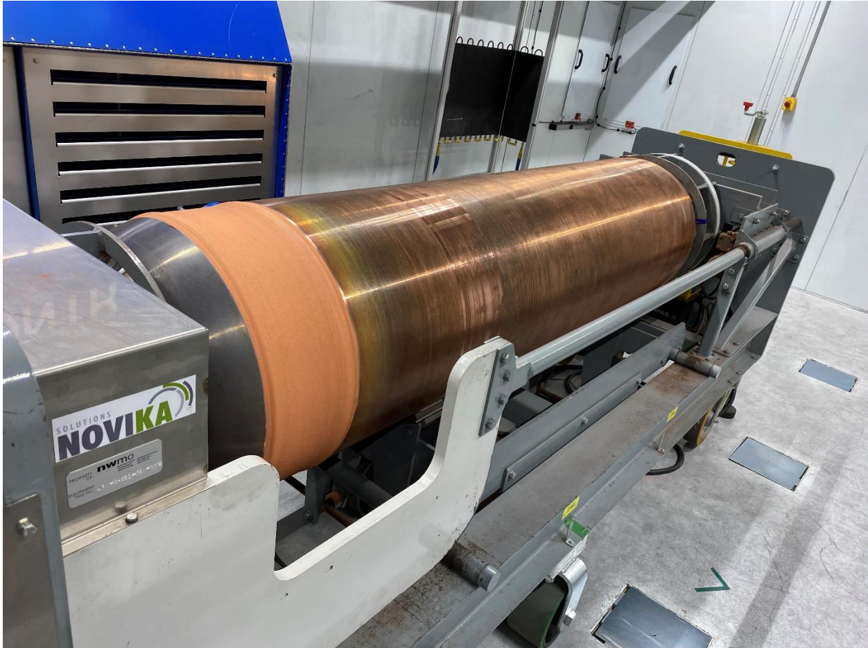
Figure 4-5: Copper Coated Closure Weld Zone on Reference Assembly UFC.
