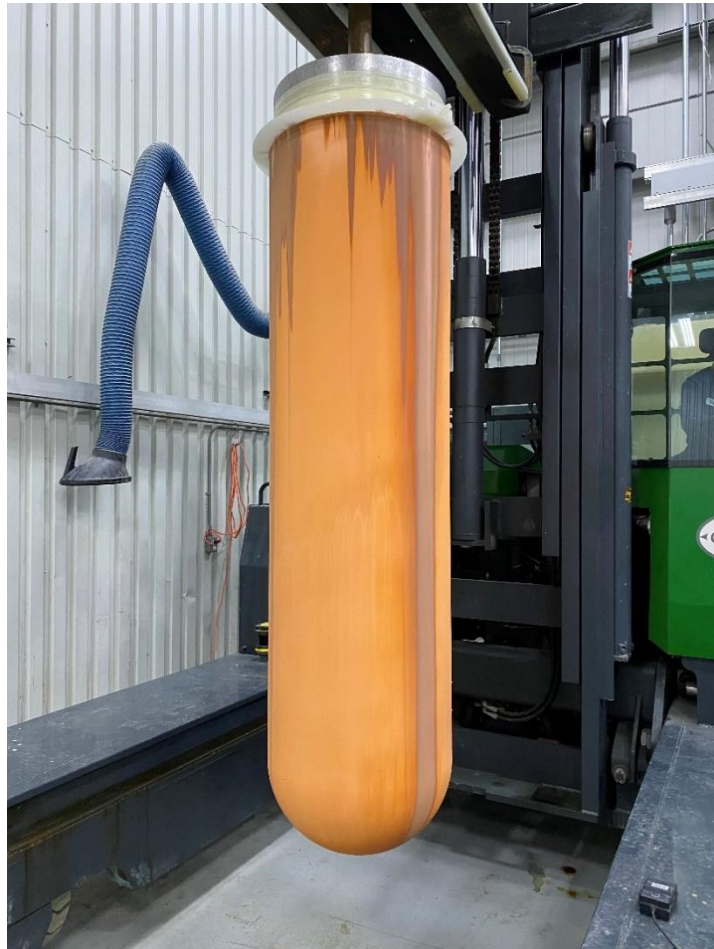
Figure 4-4: Copper Coated Serial Production Lower Assembly using Refined Acid Copper Electrodeposition Process Parameters.
