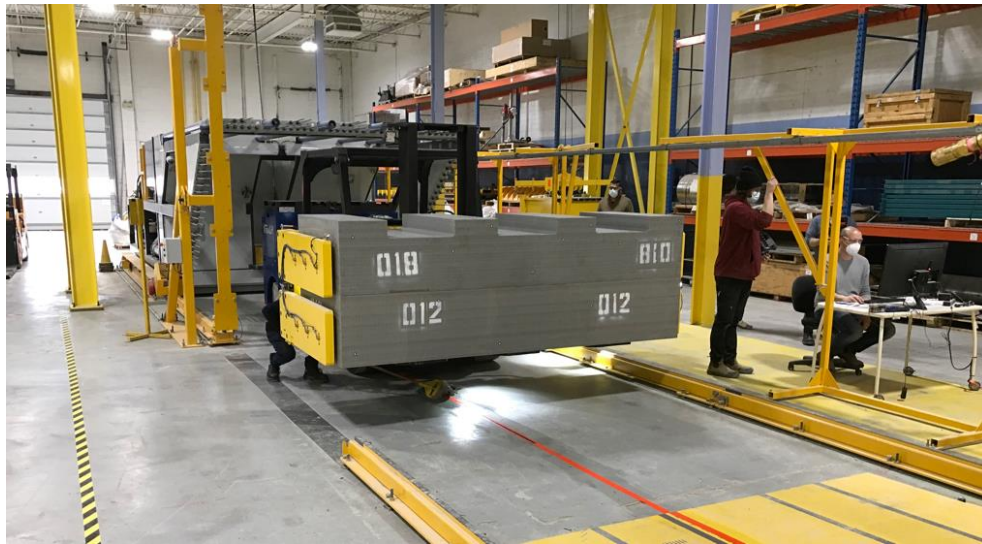
Figure 3-23: Buffer Box Delivery Equipment Ready for Delivery
