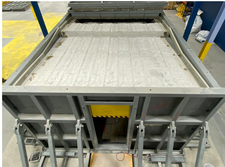
Figure 3-27: Emplacement Room Top Panels Removed
