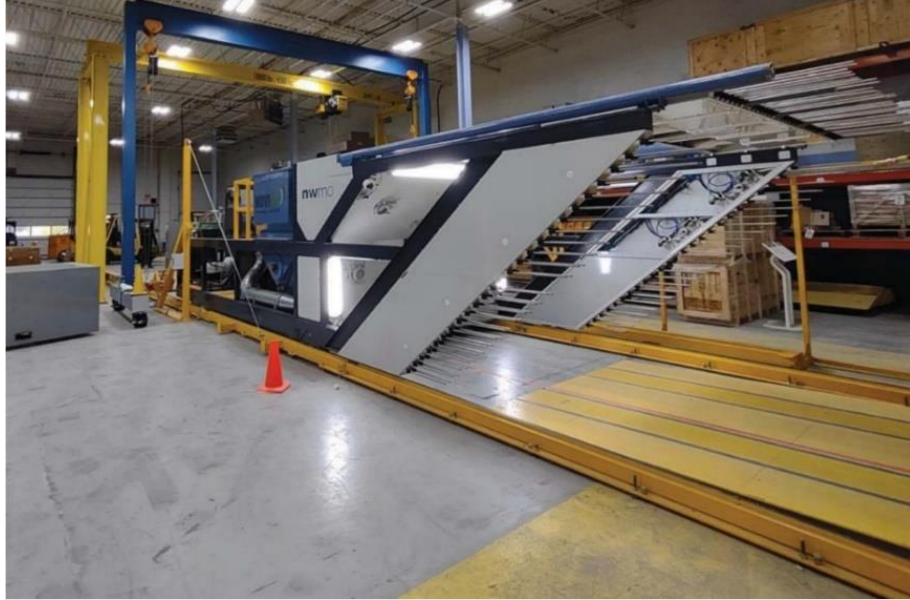
Figure 3-16: Gap Fill Material Delivery Equipment
