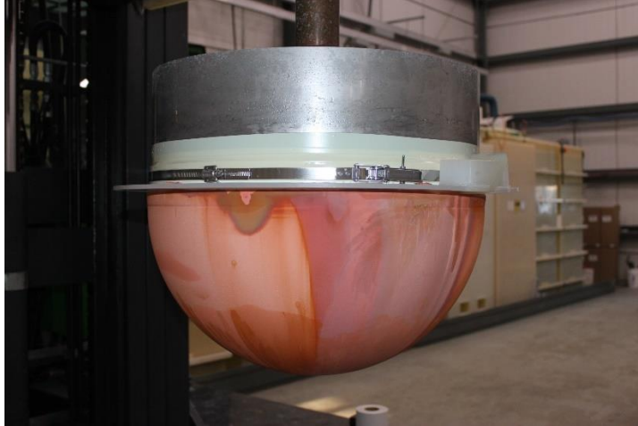
Figure 4-3: Copper Coated Serial Production Upper Hemi-head using Refined Acid Copper Electrodeposition Process Parameters.
