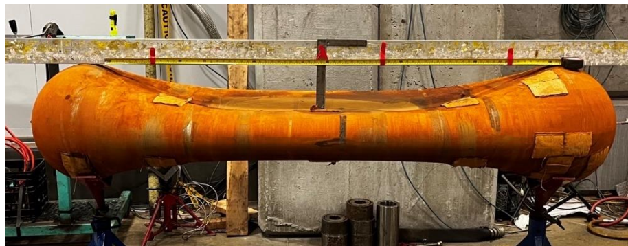
(b) Collapsed UFC After the Test
