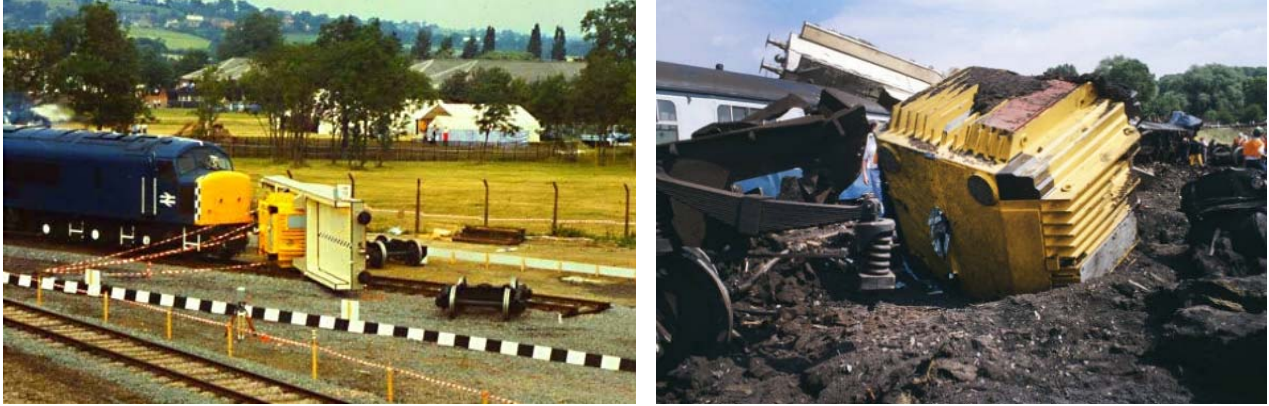
Figure 8.3: Photos from "Operation Smash Hit". A used fuel transportation package was tested by direct collision with train traveling at 160 km/h. (Left) Train just before collision, (Right) dented but intact package among wreckage.
