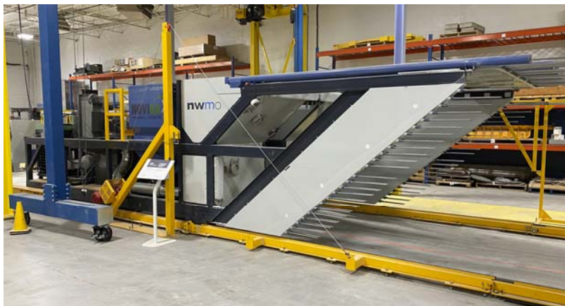
Figure 7.14: Gap Fill Material Delivery Equipment
