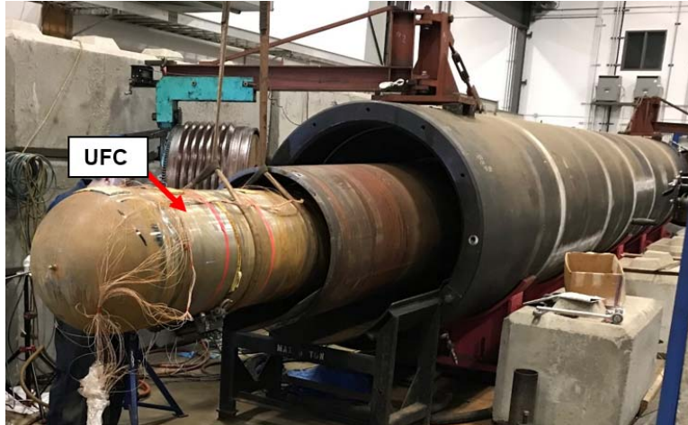
Figure 7.6: Steel prototype Used Fuel Container external pressure test at C-FER Technologies in 2022. The container is being inserted into dual-walled test chamber.
