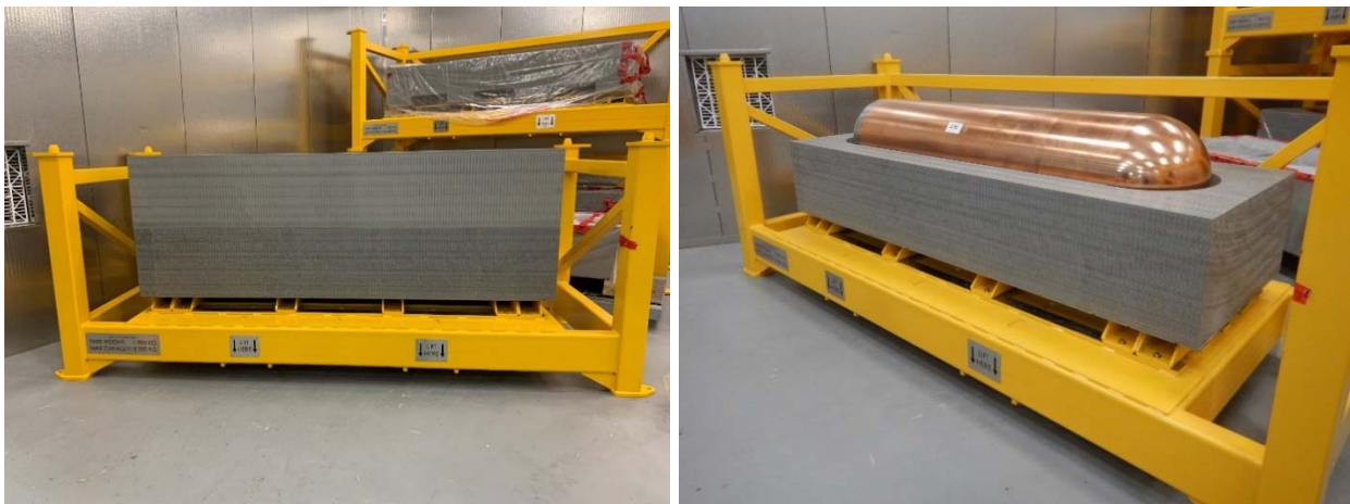
Figure 7.9: Prototype Buffer Box and Used Fuel Container
