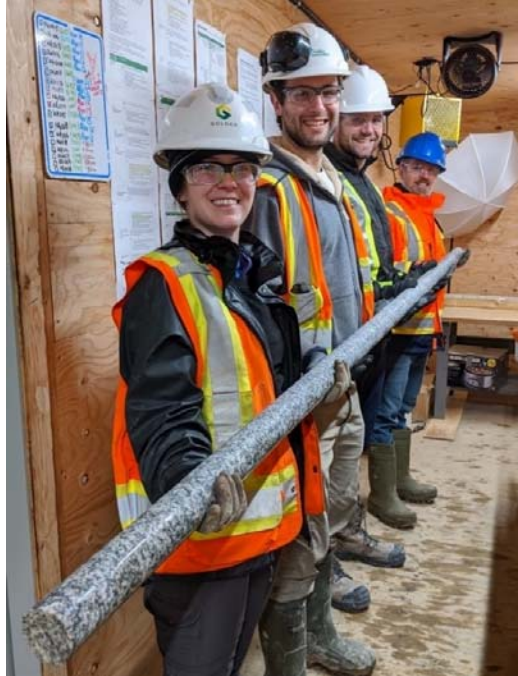
Figure 3.8: Example of an intact, three-metre long, section of drill core displaying the low fracture frequency typical of the high strength granodiorite-tonalite of the Revell Site.
