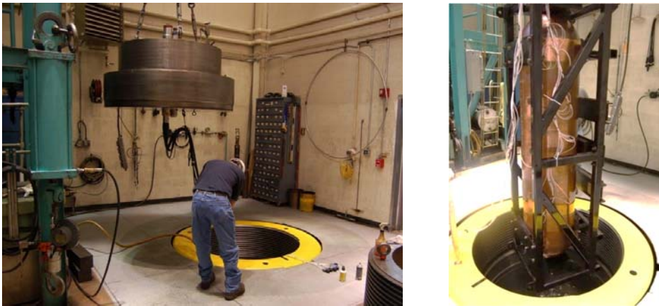
Figure 7.5: Copper coated prototype Used Fuel Container external pressure test at Penn State University in 2016. (Left) Test chamber lid being lowered into place; (Right) Container removed after experience more than 1.2 times the bounding design pressure; no significant change of configuration.
