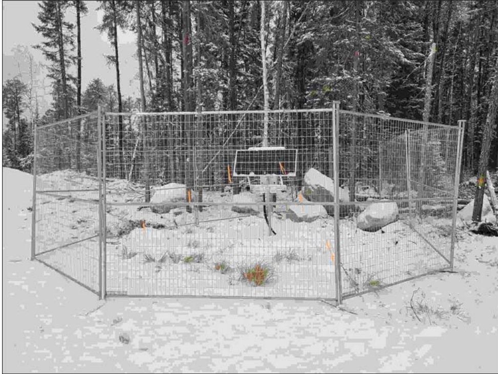
Figure 14.1: Photo of one of nine microseismic monitoring stations installed around the area in order to obtain more detailed information on site seismicity.
