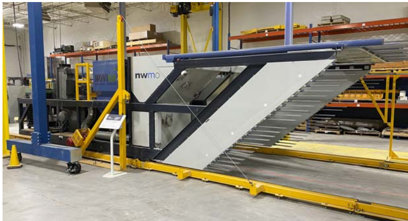
Figure 7.14: Gap Fill Material Delivery Equipment
