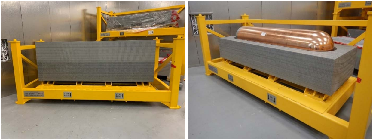
Figure 7.9: Prototype Buffer Box and Used Fuel Container
