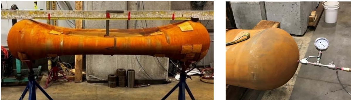
Figure 7.8: Steel prototype Used Fuel Container external pressure test. (Left) container buckled and collapsed under pressure 1.4 times the bounding design pressure; (Right) helium leak test to verify that the container is still leak tight after collapse.
