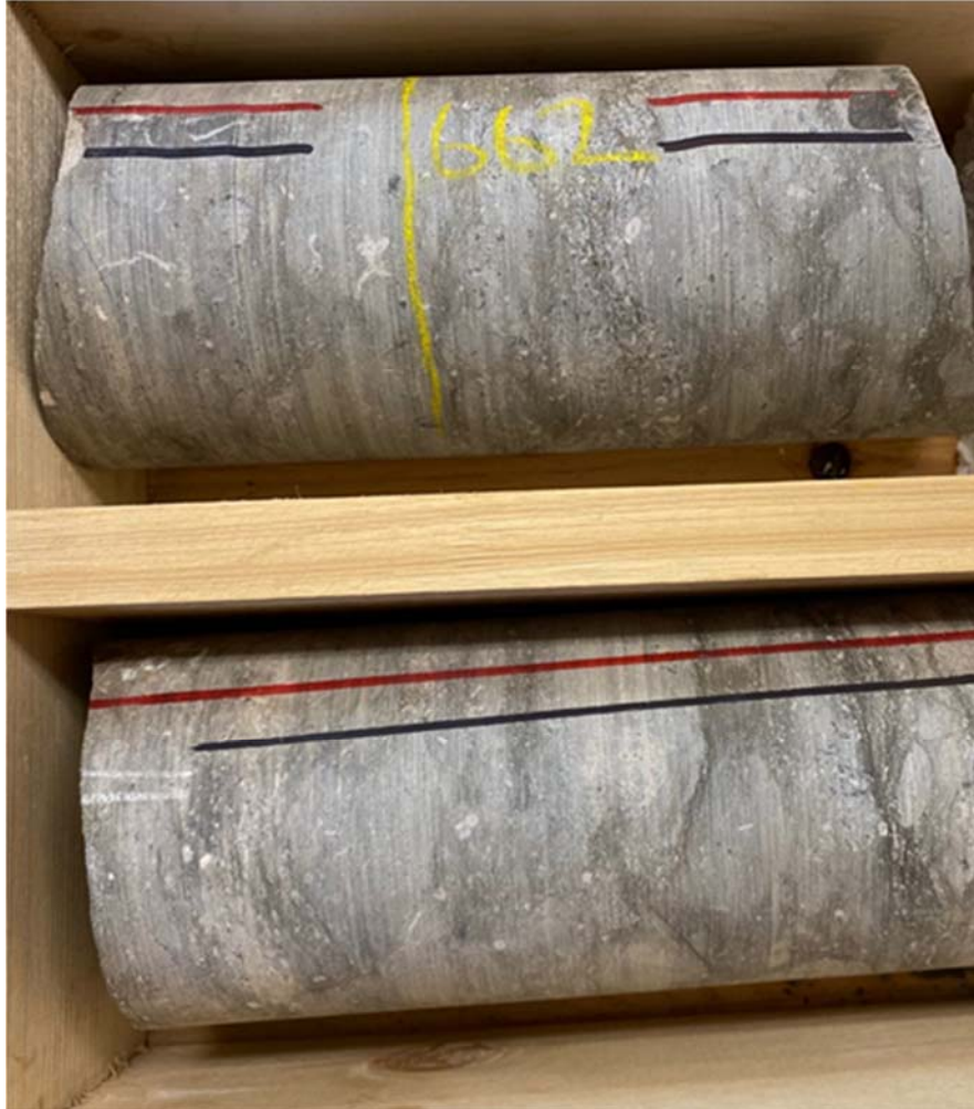
Figure 3.4: Examples of Cobourg Formation from beneath the South Bruce Site from approximate 669 m depth in SB_BH01. Each piece of core is 83 mm in diameter.
