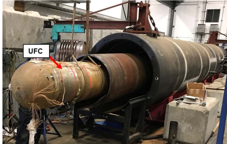
Figure 7.6: Steel prototype Used Fuel Container external pressure test at C-FER Technologies in 2022. The container is being inserted into dual-walled test chamber.
