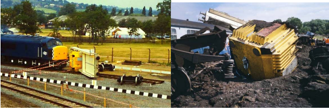
Figure 8.3: Photos from "Operation Smash Hit". A used fuel transportation package was tested by direct collision with train traveling at 160 km/h. (Left) Train just before collision, and (Right) dented but intact package among wreckage.
